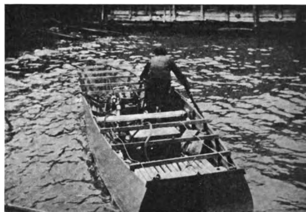
First of the M. B. C. of America's New 21-Foot One-Design Boats After a Trial Run before the Decks Were Built. We Were Aboard, and Despite a Choppy Sea and the Open Hull She Shipped no Water Aboard. See Page 282.
